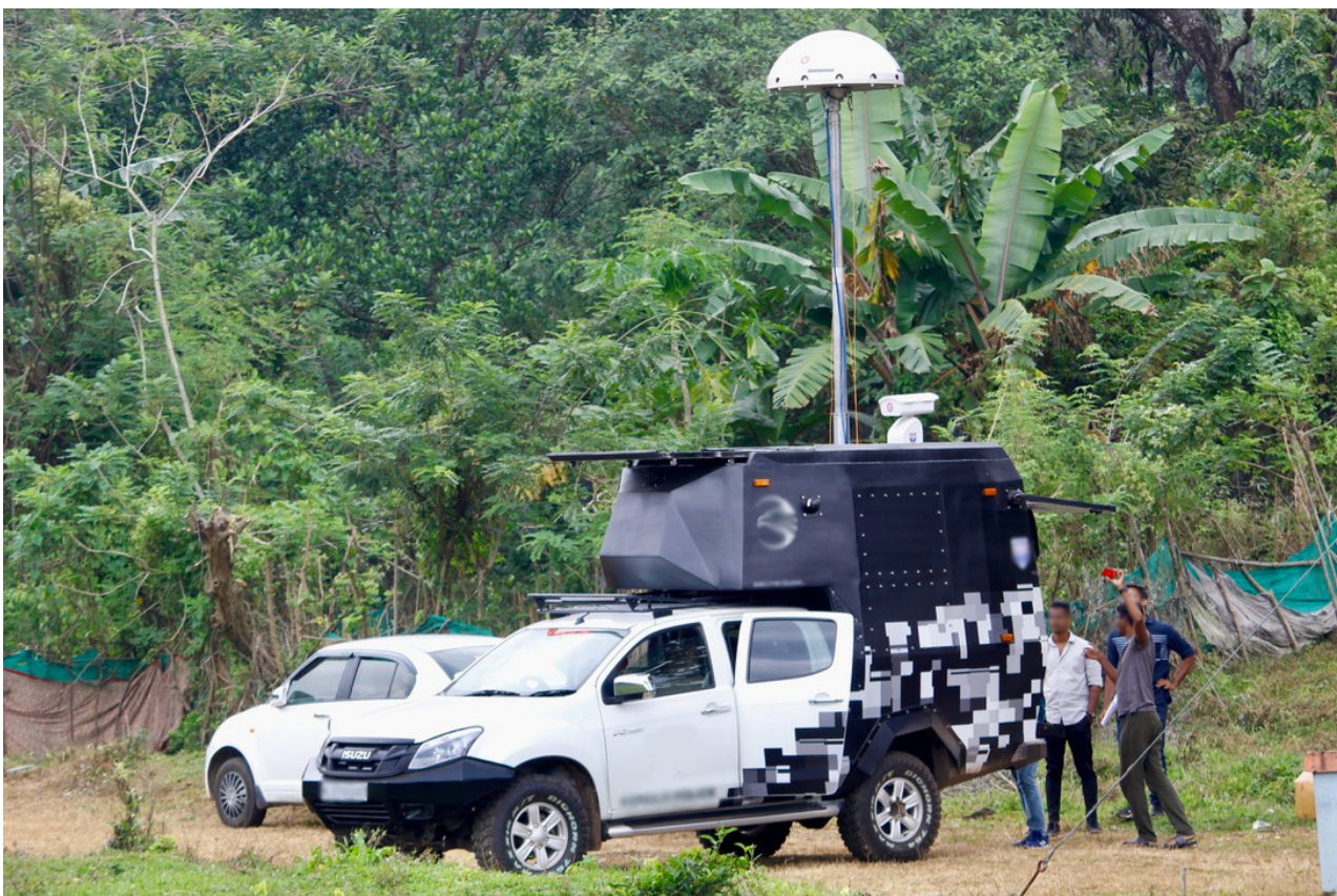
Photo: The mobile CDS field deployment. The image shows the antenna hoisted on the custom hydraulic system.
